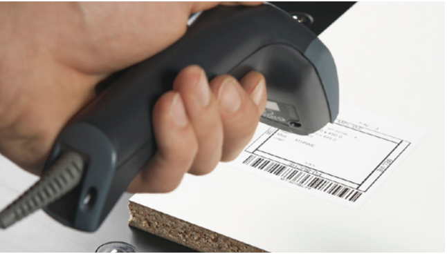
Barcode control system With the integrated barcode technology, the software makes a decisive contribution to the prevention of errors during machine operation. The unique part ID that is particularly necessary in batch size 1 production is automatically assigned by ControllerMES and is used for unique identification of components in the entire production process.
