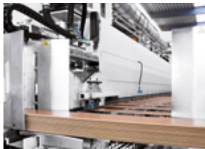
Workpiece magazine for high cycle-performance
