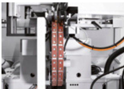
Tension-free infeed system with improved stability
