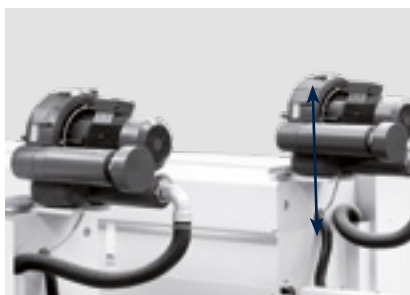
Chain track ventilation on both sides
