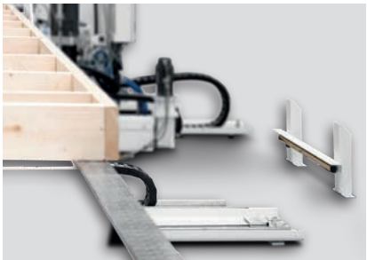
Comprehensive safety system ▪ High level of work safety thanks to protected working area with the highest safety standards ▪ Light barriers, protective fences, as well as various protective devices on the fastening units
