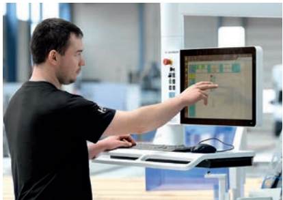
Convenient operating system ▪ Clear screen display and intuitive powerTouch user interface for easy operation ▪ Integrated data flow thanks to fully automatic data transfer from all common CAD programs ▪ tapio-ready: all the processes in the value chain combined into a single digital platform
