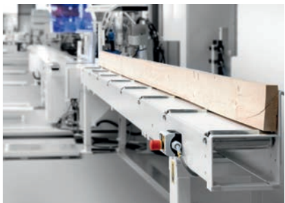
Infeed roller track Manual placement of top and bottom plates via loose, non-driven rollers.
