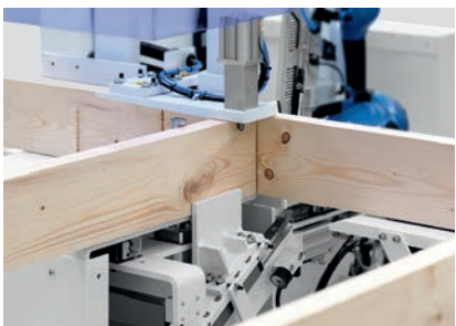
NC-controlled stopper system Specification of the placement positions of individual studs, as well as fully automatic clamping and connection of frame work. The frame work remains clamped even while the plates and studs are connected.
