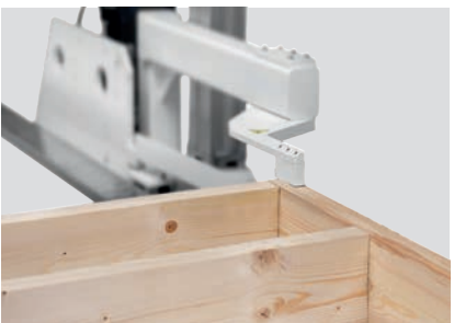
NC-controlled outfeed gripper Exact stud distances: the frame work is automatically fed to the respective placement positions.
