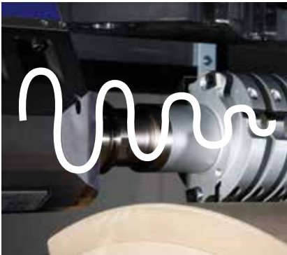
An additional vibration sensor detects tool imbalances and protects the spindle from overloads such as those caused by excessive feed rates.
