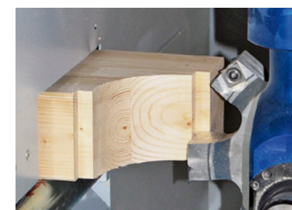
Rafter head processing
