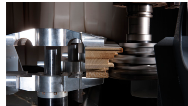
Liquid-cooled trimming spindles with vector control
