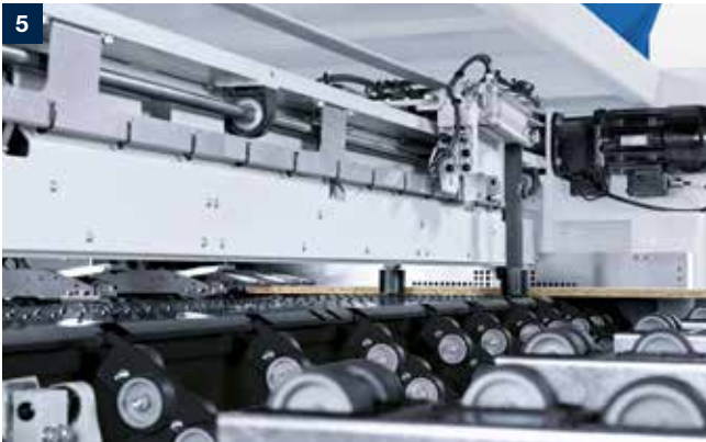
Side pressure device The SAWTEQ S-320 flexTec works with a side pressure device that is lowered from above and can be moved independently. The system presses the strips over the entire cutting length – also suitable for pressure-sensitive panels.
