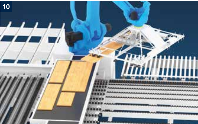
Ejecting device Automatically pushes the cut parts from the cutting line to the front machine table and thus back into the work area of the robot. Waste is removed via the waste flap.
