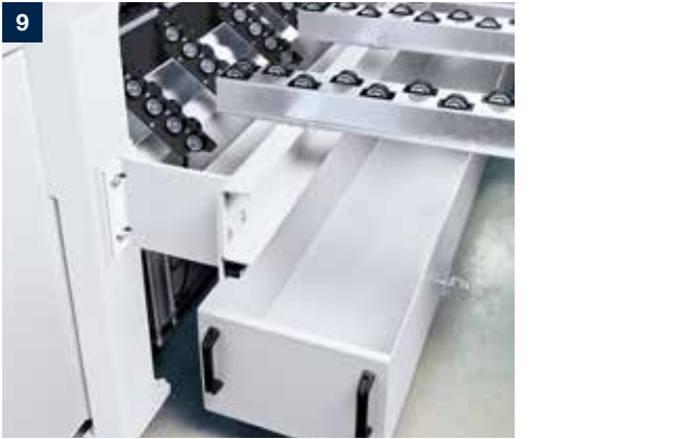
Waste disposal The waste flap opens and closes in the work cycle of the cutting cell; operation is fully automated and software-controlled.
