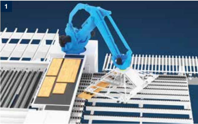
Robot with suction traverse At the heart of the SAWTEQ S-320 flexTec is a tried-and-tested industrial robot with a specially developed suction cross rail. The robot is responsible for all handling of panels, strips and parts. This is fully automatic, highly flexible, error-free and efficient.
