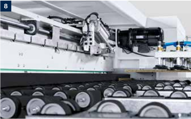
Ejecting device Automatically pushes the cut parts from the cutting line to the front machine table and thus back into the work area of the robot. Waste is removed via the waste flap.
