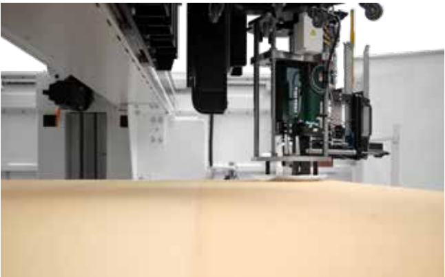
Glider The glider can be used to attach soft wood fiber boards without damaging the material.
