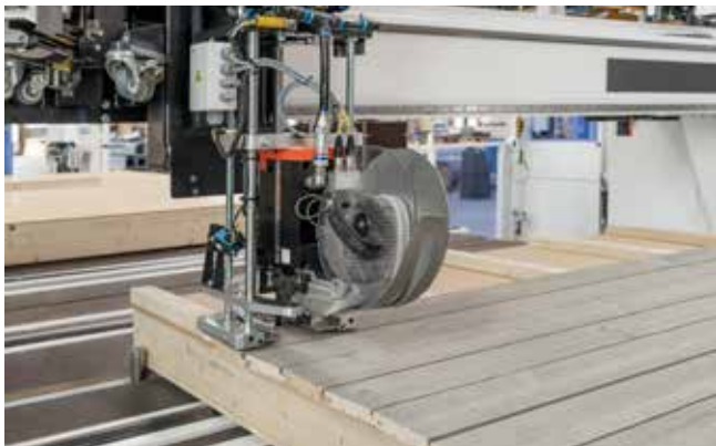
Facade shoe The facade shoe makes it possible to attach and format wooden facades semi-automatically.
