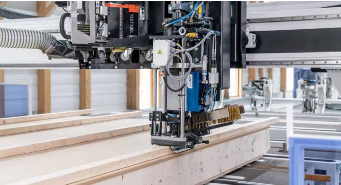
Batten shoe The batten shoe can be used to increase the degree of automation in the prefabrication of roof elements. The battens can be attached semi-automatically.
