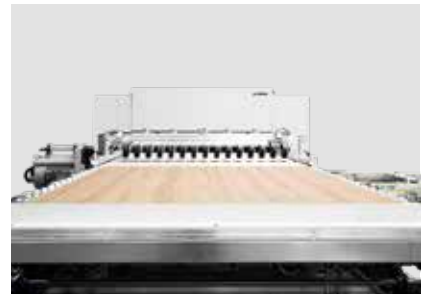
Rip cut panel dividing
