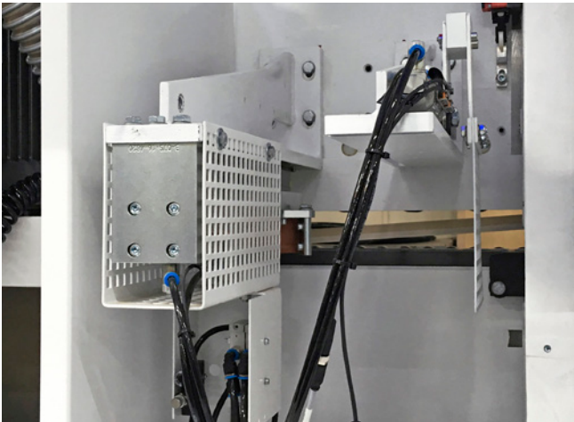
Safety pressure device For grooving in solid wood strips in synchronous operation.
