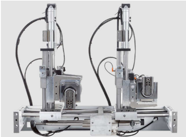
MF50 multifunction trimming unit For processing edge overhangs on the upper and bottom edge of the workpiece and copying of the corners of the front and rear edge. Equipped with automatic adjustment between thin and thick edges. Workpiece thickness 60 mm.
