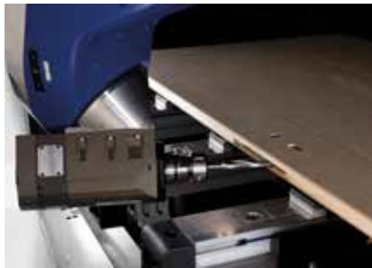
Trimming the lock casing
