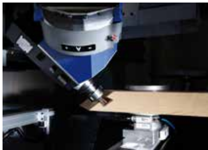
Trimming a burr connection for jamb/rail designs
