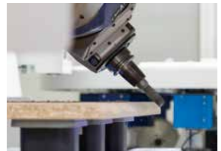
Traced flush milling of the edge overhangs on the postforming profile
