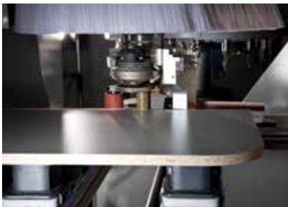
easyEdge gluing unit for rational gluing on shaped parts
