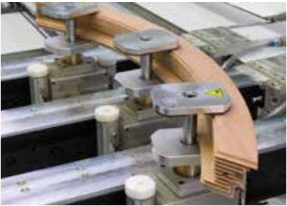
3-step clamp: Highly rigid 3-step clamps with extreme clamping height for precise complete processing of window and front door components without subsequent outside moulding and profiling.
