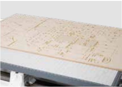
Matrix adapter plate also offers secure fixing for filigree workpieces. Shaped parts in the nesting process can also be “tailored” on a console table in an optimized way with the matrix adapter plate.
