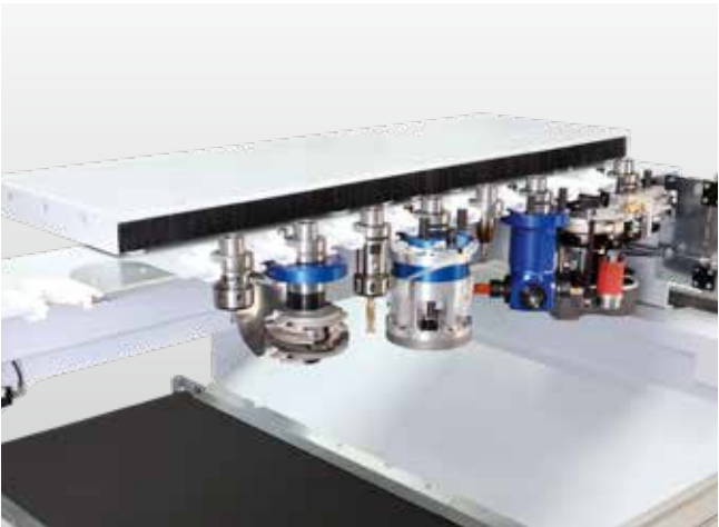
8-fold linear changer with tool transfer station, mounted on the side. As an option, the pick-up station for the easyEdge unit can also be integrated.
