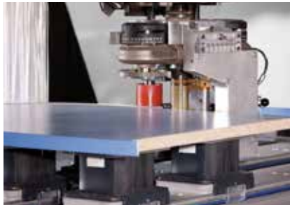
easyEdge edge banding unit is the universal solution for edging small quantities.
