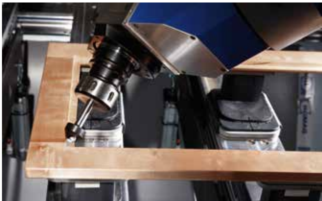
Angular cutting of a glass rabbet corner
