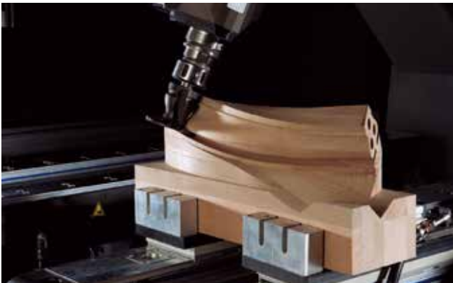
Routing a staircase handrail
