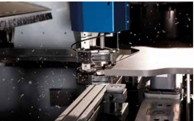
Perfect edge finish through traced combination flush routing/scraping unit
