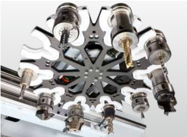
10-fold tool changer traveling with spindle. Tool change during drilling or edge banding. For tools and units with a diameter of up to 180 mm.
