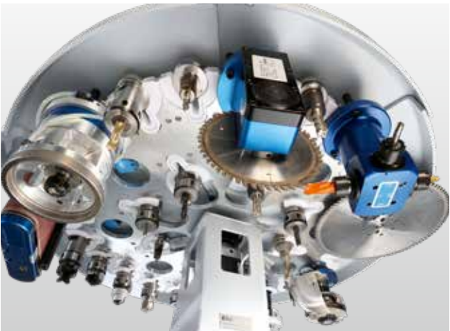
32-fold tool changer – arrangement of the tools in an inner and an outer ring. For tools and units with a diameter of up to 200 mm and saw blade up to 350 mm in diameter (in the outer ring).
