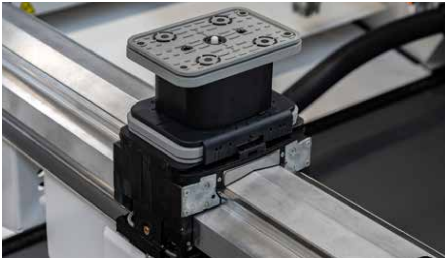
Vacuum clamps with tracing valve – unoccupied suction cups can remain on the platform. Mounting height 100 mm
