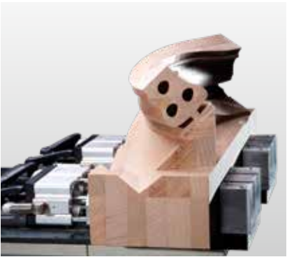
Clamping unit ensures safe and quick clamping of jambs and scantling.
