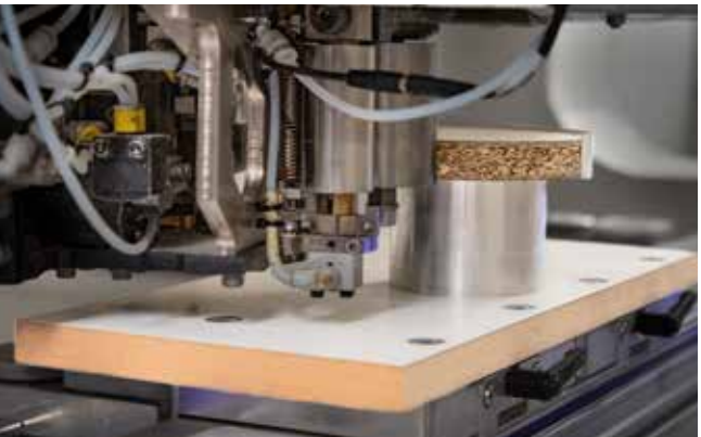
360° edge gluing with the powerEdge Pro Duo edge banding unit
