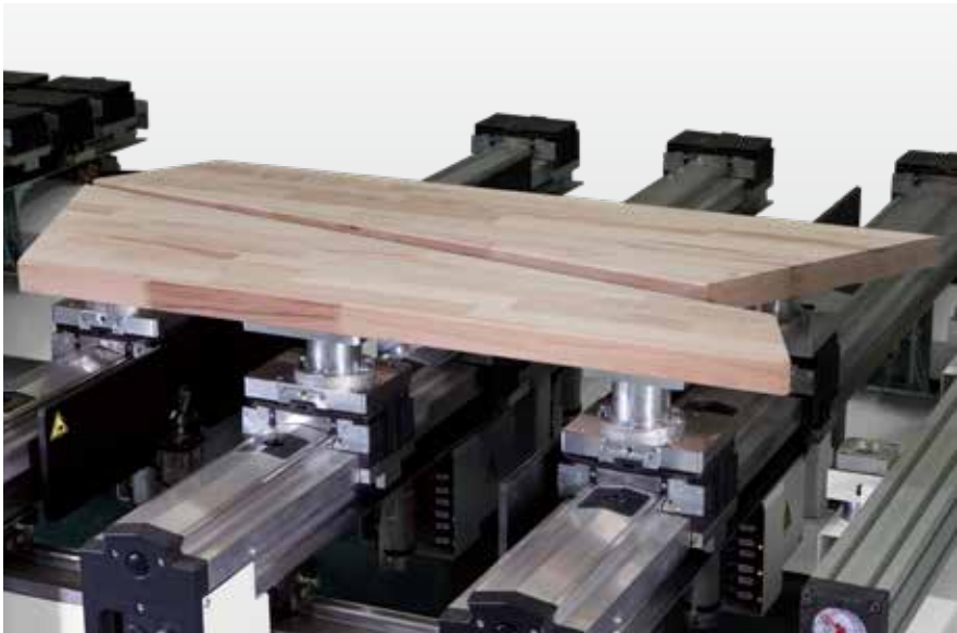
movePart ensures automatic moving apart after separation in the program sequence for complete processing.
