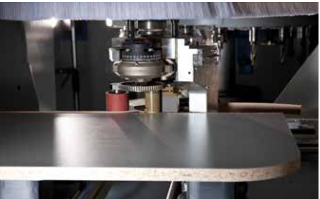
easyEdge gluing unit for rational gluing on shaped parts
