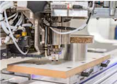
powerEdge Pro Duo edge banding unit – one unit for all requirements. Zero joint technology and accurate tracing ensure perfect results for 360° gluing.
