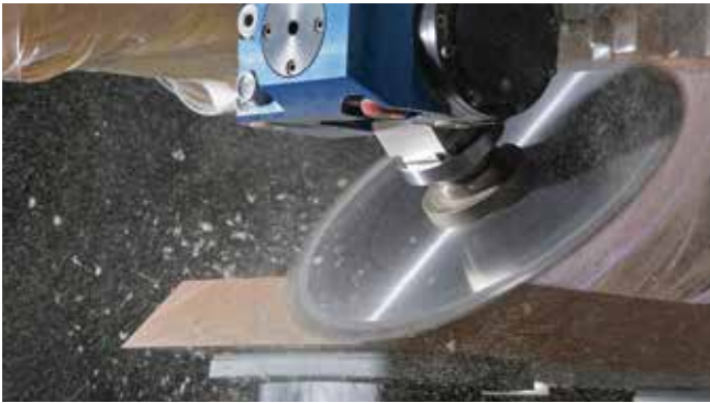
Sawing, routing, drilling at any angle – FLEX5+ unit with automatic angle adjustment and automatic tool change. A unique unit for 4-axis spindles, which covers over 90% of 5-axis applications.
