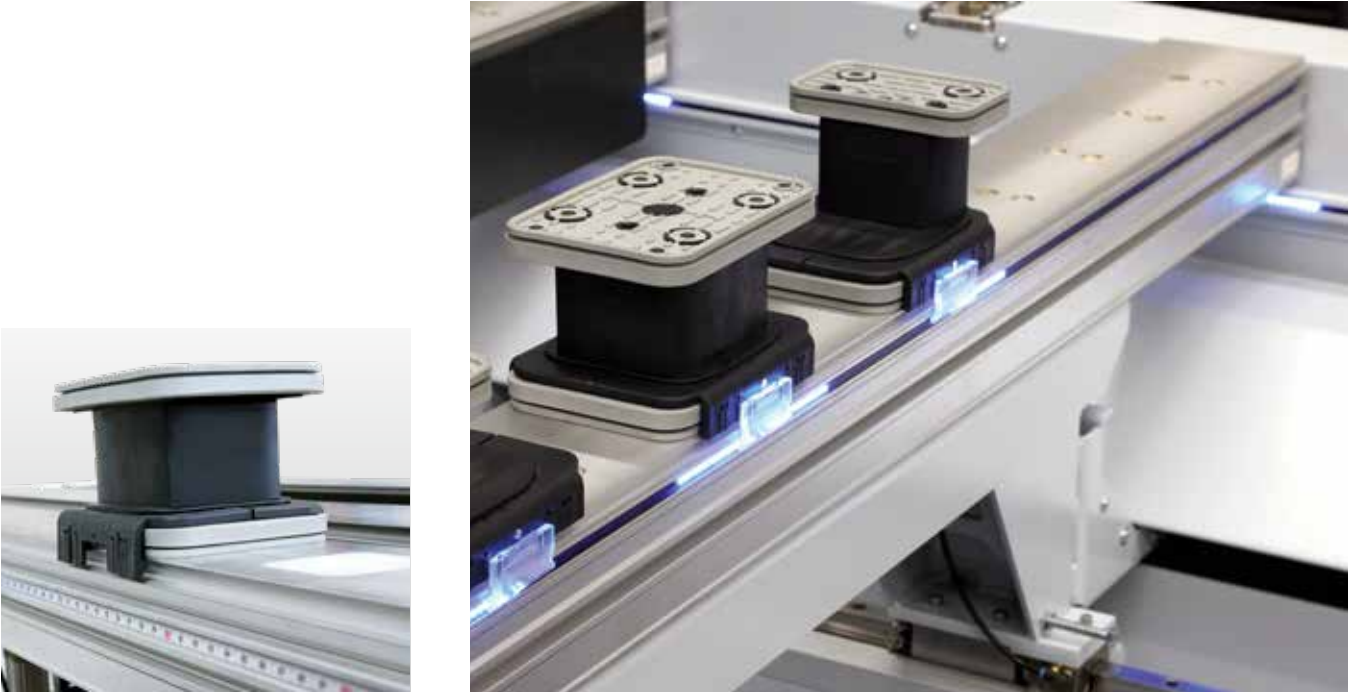
Measuring tape for positioning the suction units.
