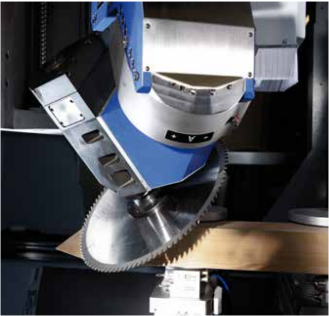
5-axis routing spindle DRIVE5CS/C+ with 10 kW of power (optionally 12 or 15 kW) and a controlled spindle speed from up to 24,000 rpm for a high torque even at low engine speeds.
