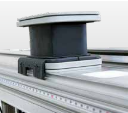
Measuring tape for positioning the suction units.
