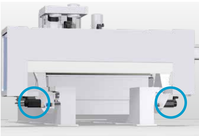
Synchronous drive 2 synchronised digital servo-drives in X-direction guarantee highest precision
