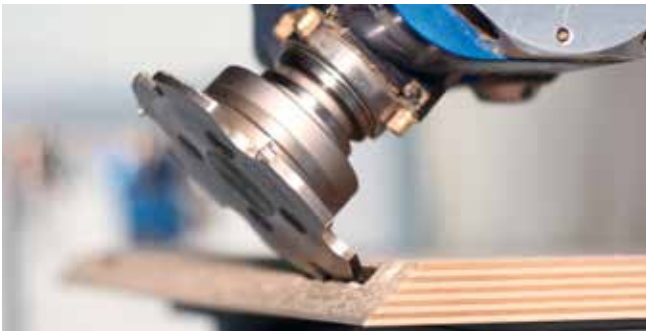
Cutting recesses for connecting fittings
