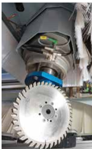
C-axis (0-360°) for the use of units
