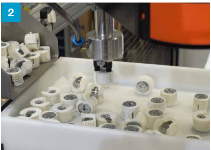
The vibrating plate rotates the connectors into the correct position
