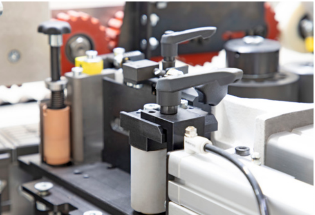
Roller counterpressure Roller counterpressure for sensitive edge material.
