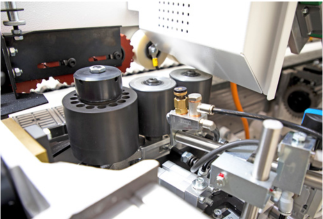
Pressure zone Heavy pressure zone up to 8 mm edge thickness and 60 mm panel height for optimum glue joint quality.
