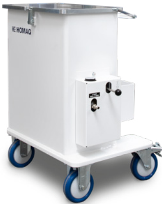
Vacuum container ▪ Compact, portable tank for the bottom application unit which is filled with PUR glue. ▪ No vacuum pump required (Venturi nozzle), as the vacuum is generated via the connection to the compressed air supply in your workshop. ▪ No nitrogen is necessary due to storage in a vacuum.
